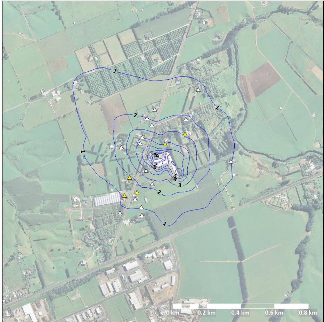
Figure 1: Spatial distribution of 99.5 th percentile 1-hour average odour concentrations associated with the proposed operation (including change to free range configuration and installation of roof vents). Submitter dwelling locations are denoted in yellow, other dwelling location in white
