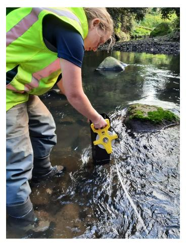
**Photo 2** Monitoring of suspended fine sediment by black disk visual clarity.
