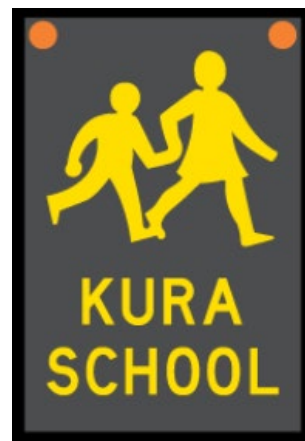
Example of Kura School warning sign (illuminated when activated)
