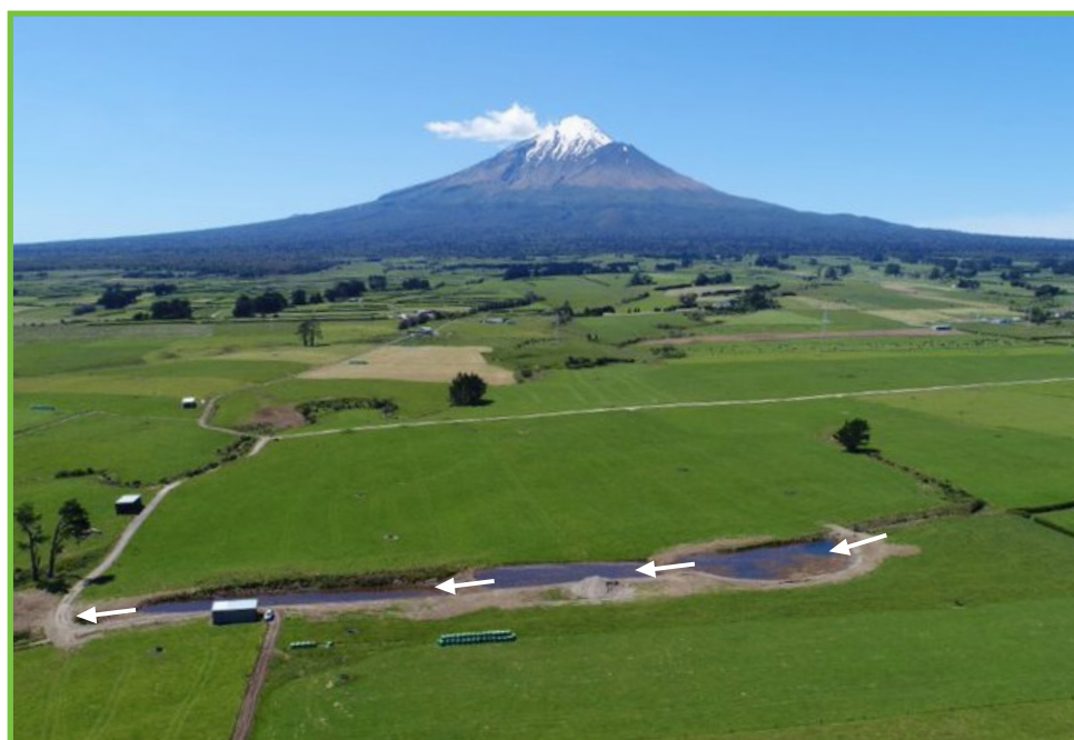
Newly constructed and planted wetland (left) showing direction of flow through initial deep sedimentation pond and subsequent two shallow elongated cells. Plant cover after one year shown on the right.
