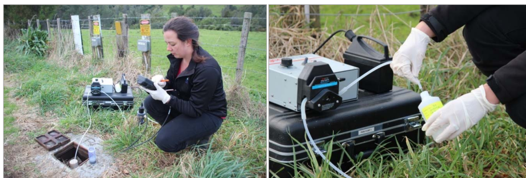
Figure 1A Groundwater bore GND0508 is continuously monitored while purged of standing water using a peristaltic pump purging. Groundwater sample is collected when field parameters are stabilised
