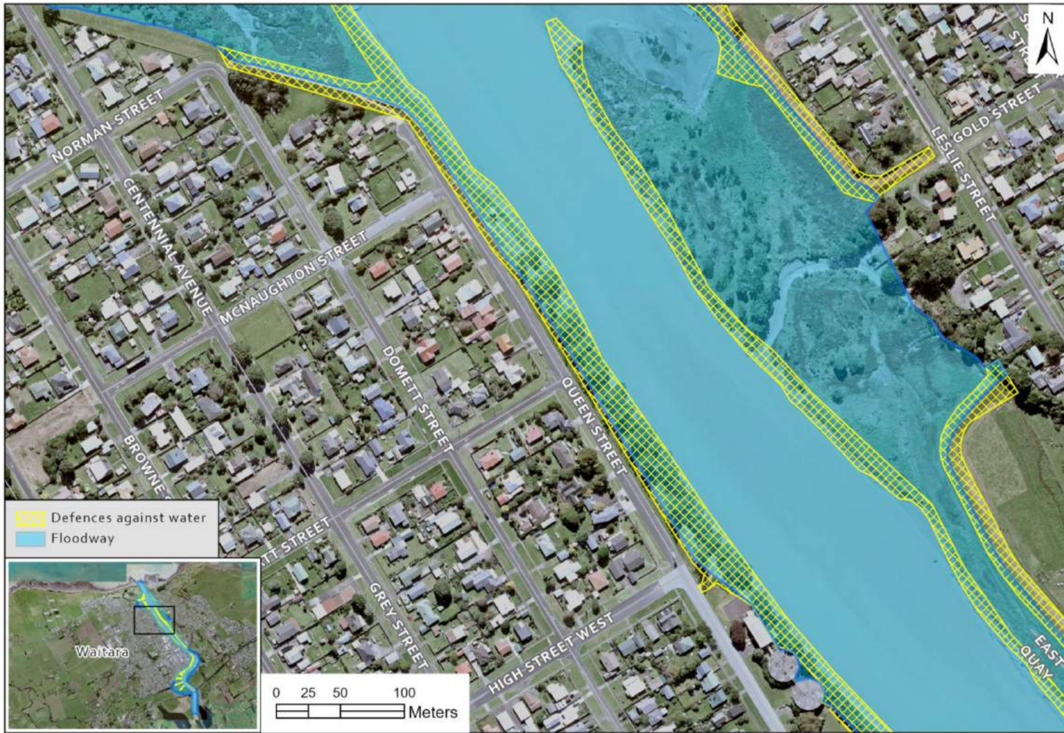
Map 2b Defences against water and floodways along the Waitara River, New Plymouth.
