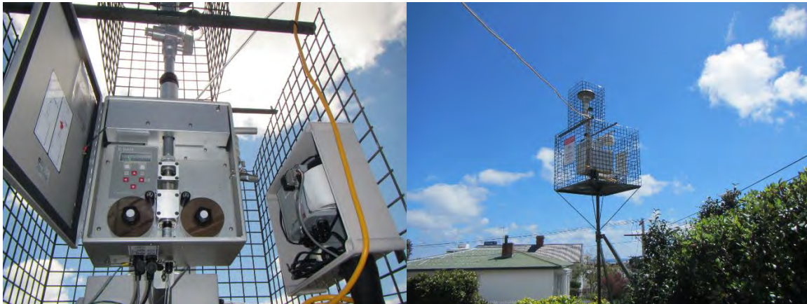
Figure 5 E-BAM set-up and installation at Central School, New Plymouth
