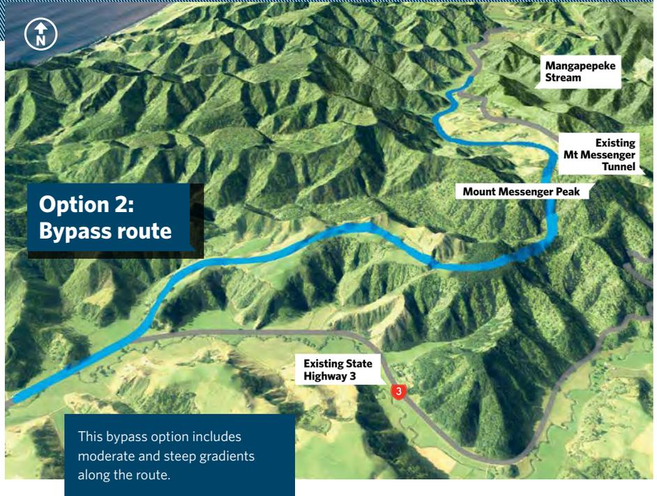
This option provides a likely speed limit of 60 to 70km/h and passing lanes uphill in both directions.
