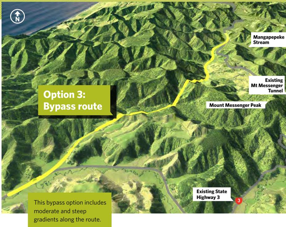
To get through the hills and valleys the route includes some very high cut slopes (up to 120 metres high) and areas built up by about 50 metres from the existing ground level to new higher levels.
