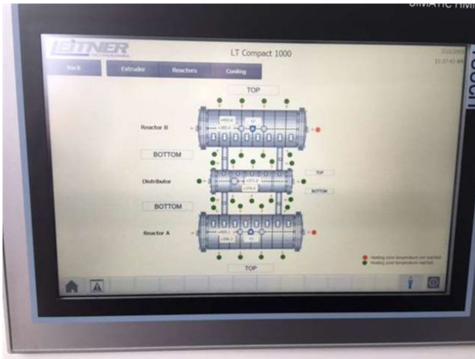
Figure 6: Monitoring the Process
