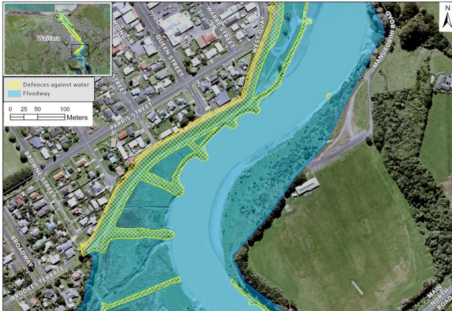
Map 2d Defences against water and floodways along the Waitara River, New Plymouth.
