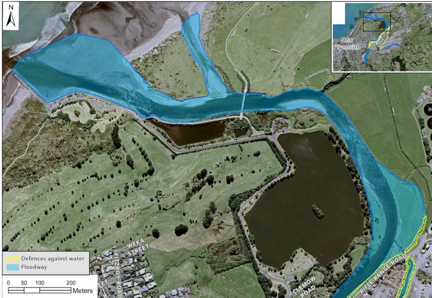
Map 3a Defences against water and floodways along the Waiwhakaiho River and Upper Mangone Stream, New Plymouth.
