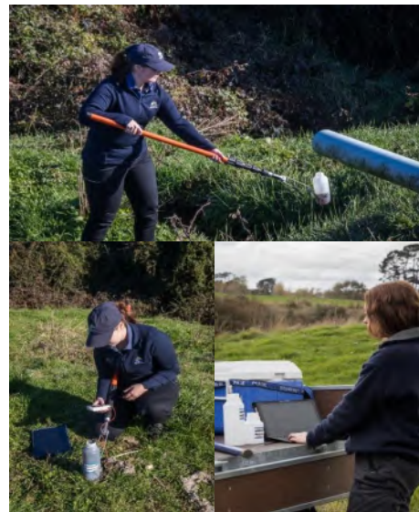
Photo 3 Collecting samples, recording temperature and entering sample information into the laboratory database remotely
