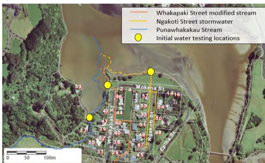
Figure 1 The Lower Urenui Township, with the Punawhakakau Stream (blue), Whakapaki Street modified stream (orange) and Ngakoti Street stormwater network (yellow). Sample locations shown as yellow dots.
