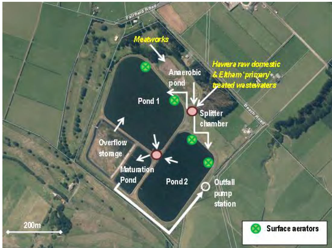
Figure 2: Configuration of the treatment system at the HWWTP
