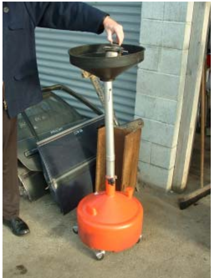
Photo 2: Fluids should be drained from old parts and correctly disposed of
