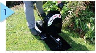
Pull back firmly on the trap setting handle. With a stick, push down on the treddle plate - keeping grip of the setting handle. Slowly reclose the handle.
