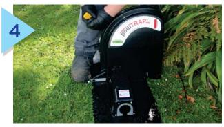
Put your foot on the front screws and pull the setting arm all the way back. Slowly move the setting arm forward until you feel it load on the catch.
