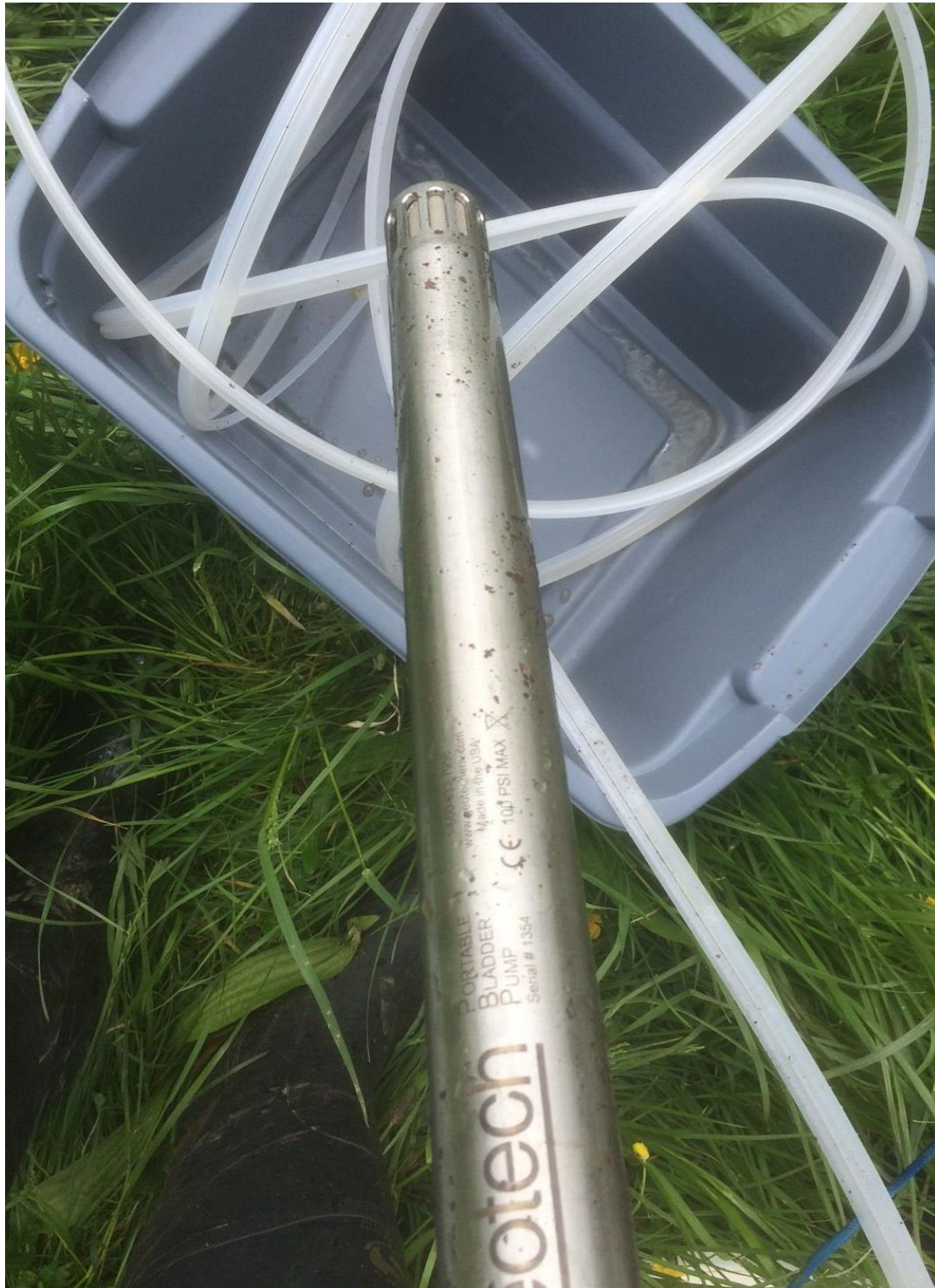
Figure 6.1: Bladder pump post sample collection in GND 2705
