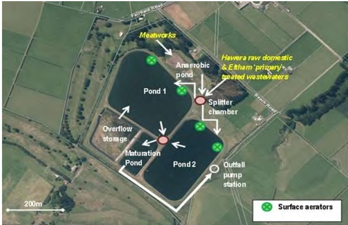
Figure 1 Configuration of the HWWTP (adapted from NIWA, 2012)
