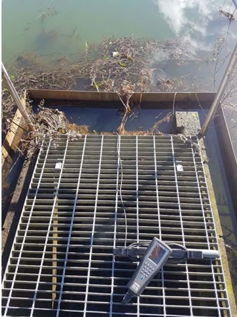
Photo 3 Dissolved oxygen monitoring
