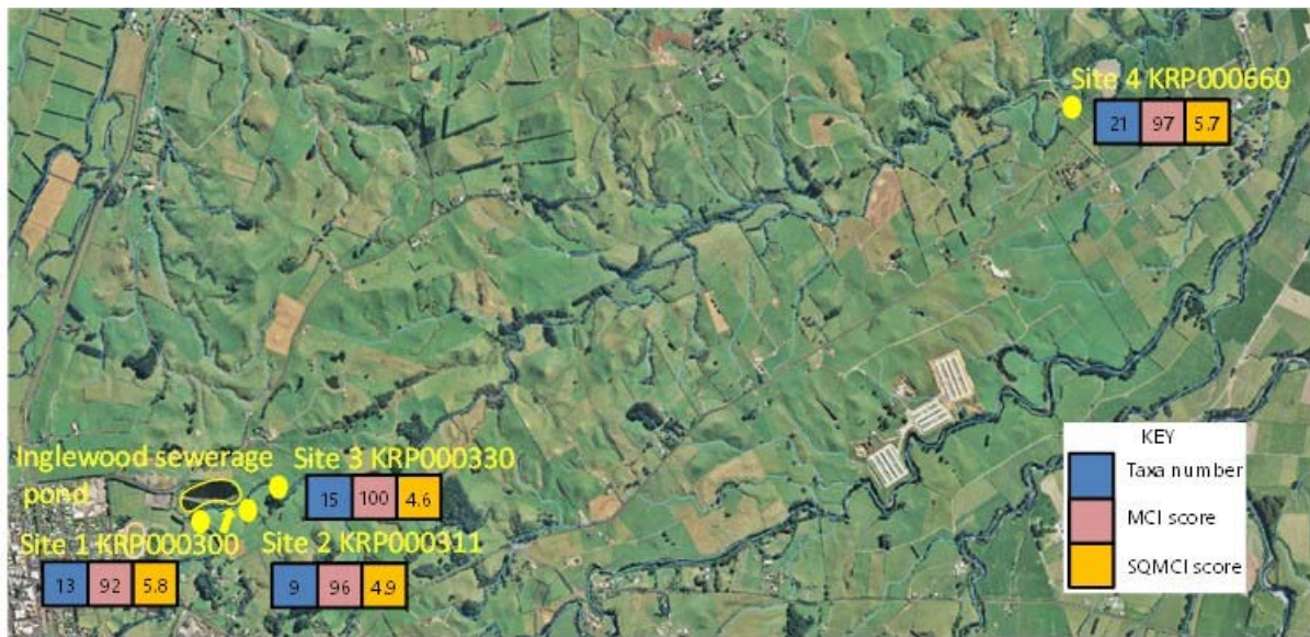
Figure 1 Sampling sites in the Kurapete Stream in relation to Inglewood oxidation ponds with taxa number, MCI scores and SQMCI scores for each site
