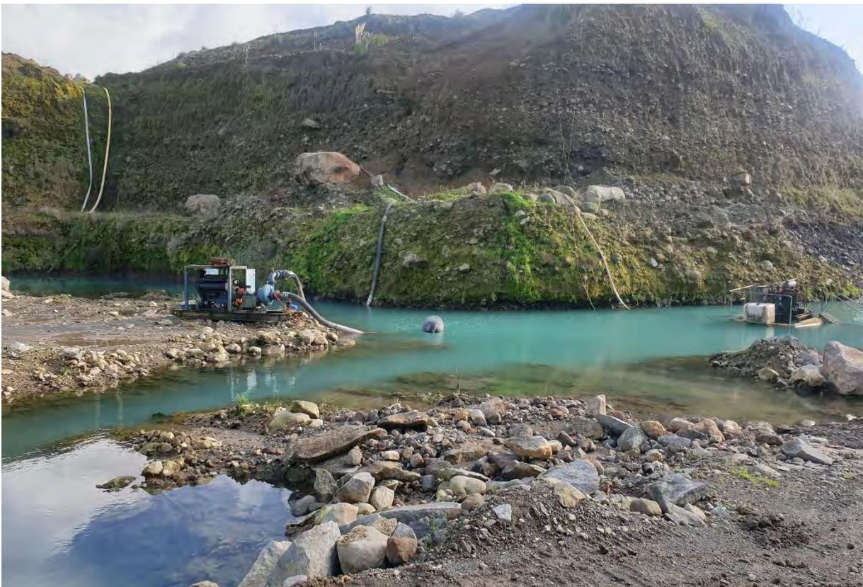
Photo 4 Ferndene Quarries Ltd groundwater seepage being pumped to the stormwater ponds, May 2019
