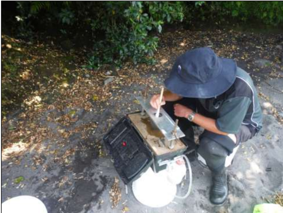
Photo 3 Device used to extract periphyton for chlorophyll a analysis. Periphyton was scrapped off the rock using a stiff paint brush. The tube at the side is used to suck up fine particles of periphyton
