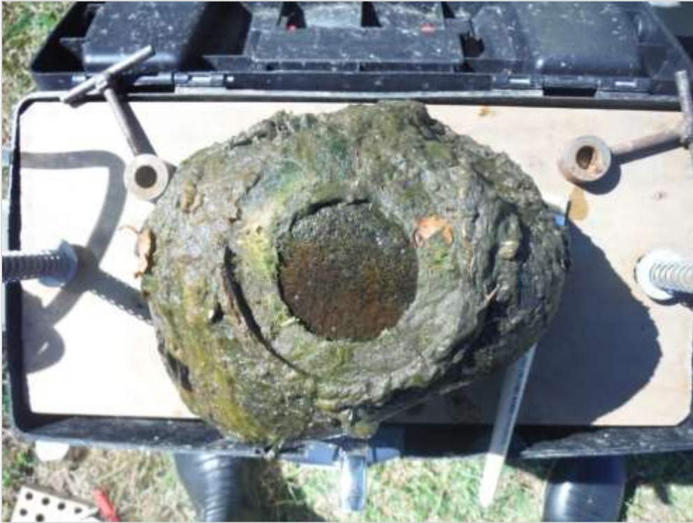
Photo 4 Periphyton covered rock with clear area where all the periphyton has been extracted for chlorophyll a analysis
