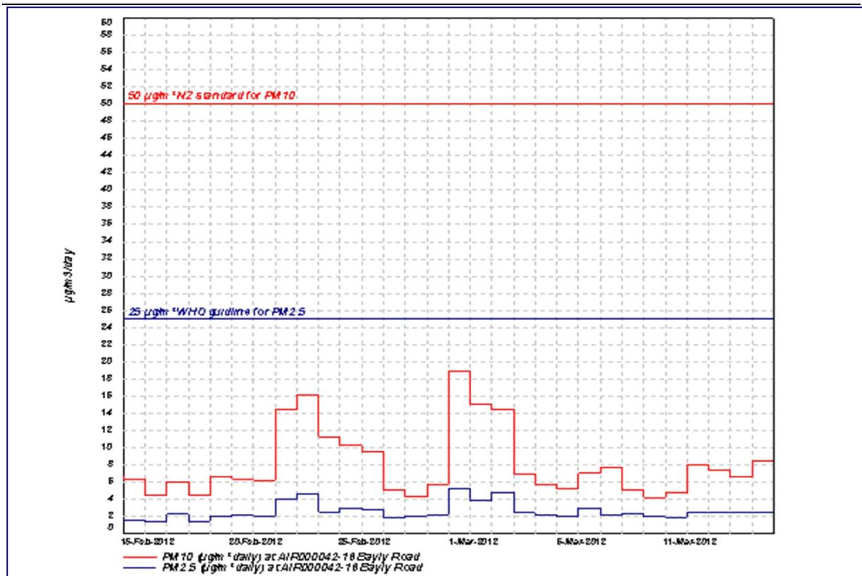
**Figure 2** PM10 and PM2.5 concentrations ( $\mu\text{g}/\text{m}^3$ ) at Bayly Road (Port Taranaki)
