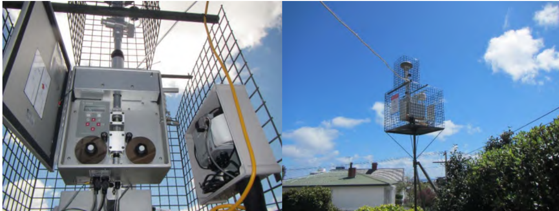
Figure 4 E-BAM set-up and installation at Central School, New Plymouth
