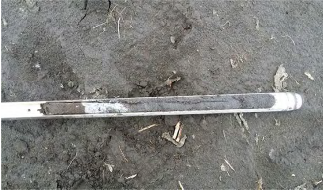
Photo 1 An example of an extracted soil core
