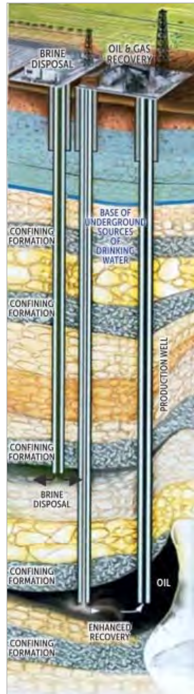
Figure 1 DWI schematic ( www.epa.gov/uic )
