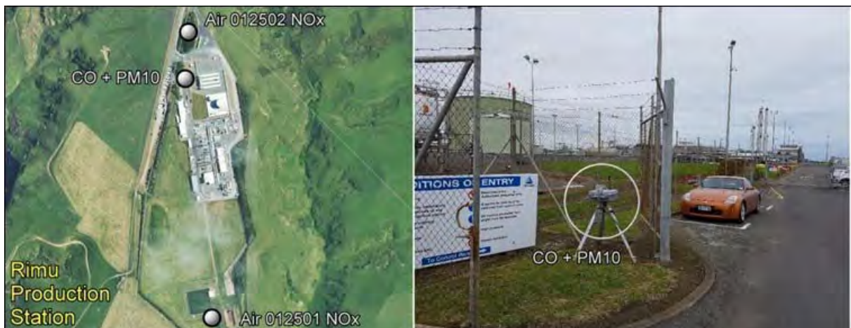
Figure 1 Air monitoring sites at Rimu Production Station for 2017-2018
