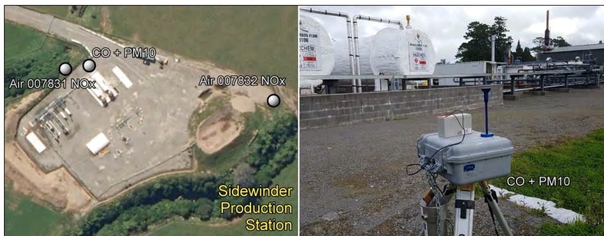
Figure 1 Air monitoring sites at Sidewinder production station (2016-2017)
