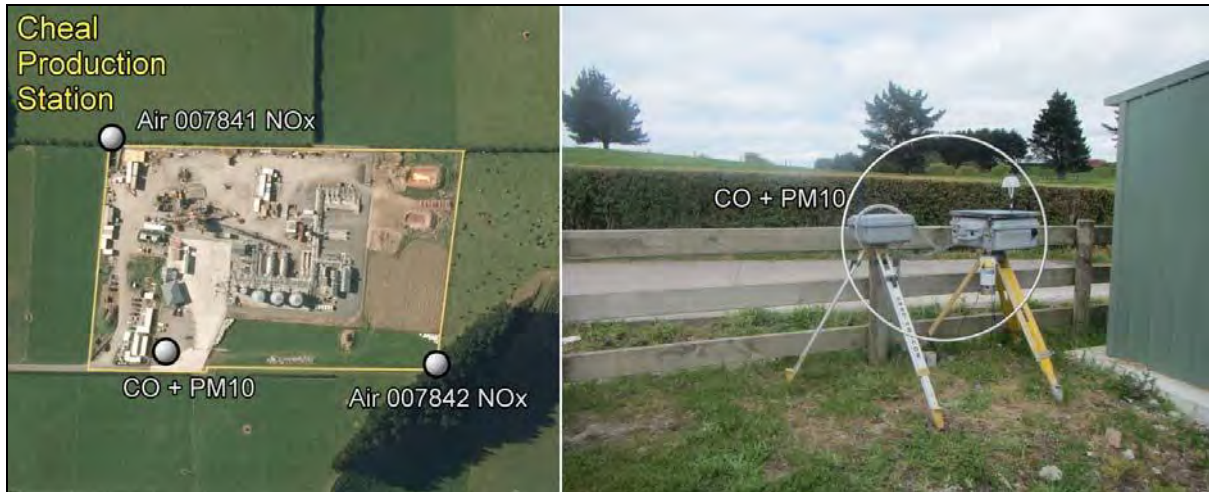
Figure 1 Air monitoring sites at Cheal production station (2015-2016)
