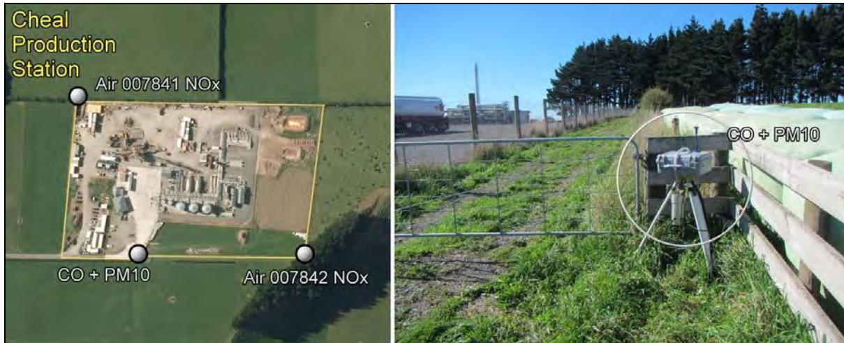
Figure 1 Air monitoring sites at Cheal production station (2014-2015)
