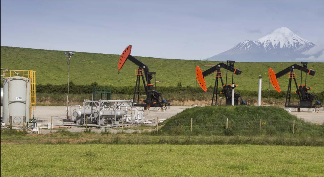
Photo 1 Pump jacks at the Copper Moki site
