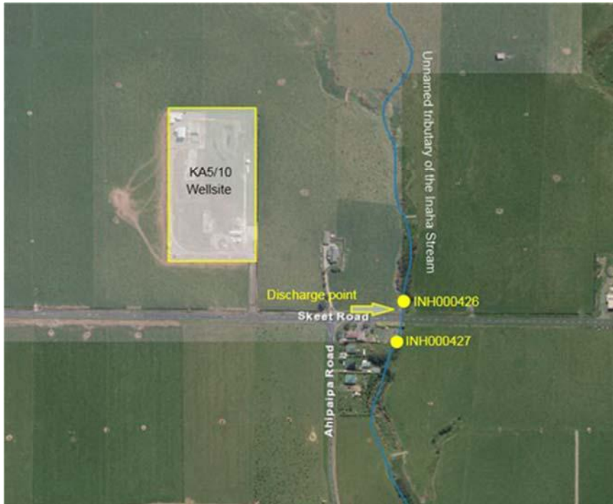
Figure 4 Biomonitoring sites in the unnamed tributary of the Inaha Stream sampled in relation to the KA5/10 wellsite
