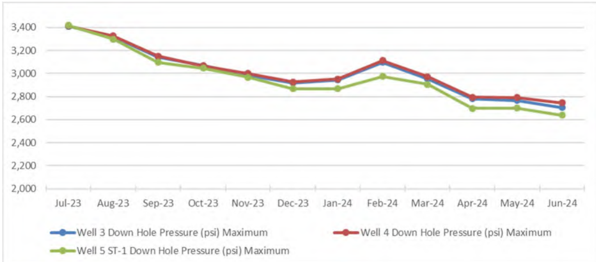
Figure 5 Monthly downhole pressure for Ahuroa B gas wells 3, 4 and 5ST-1 July 2023-June 2024
