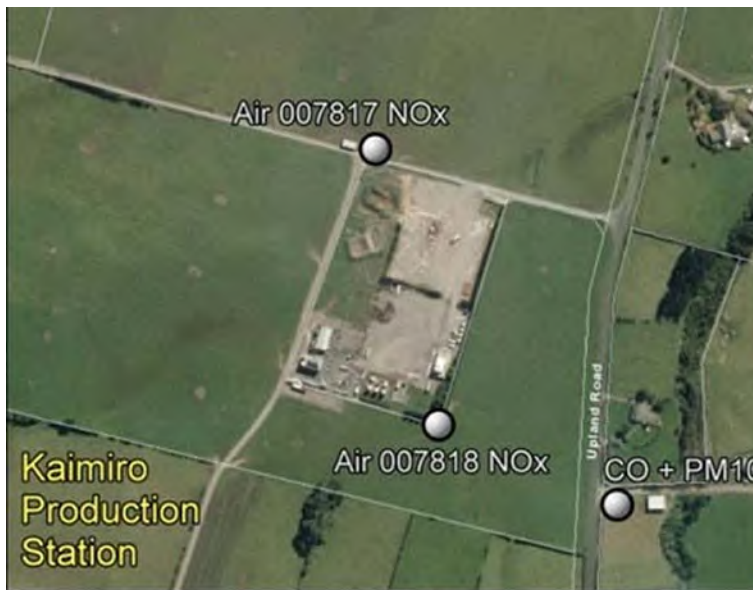
Figure 5 Air monitoring sites at Kaimiro Production Station
