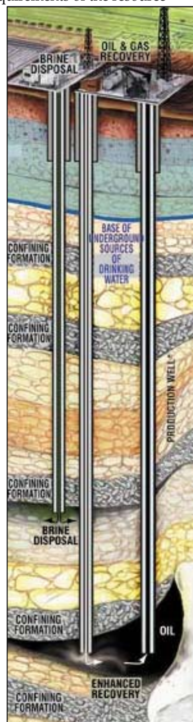
Figure 1 DWI schematic ( www.epa.gov/uic )
