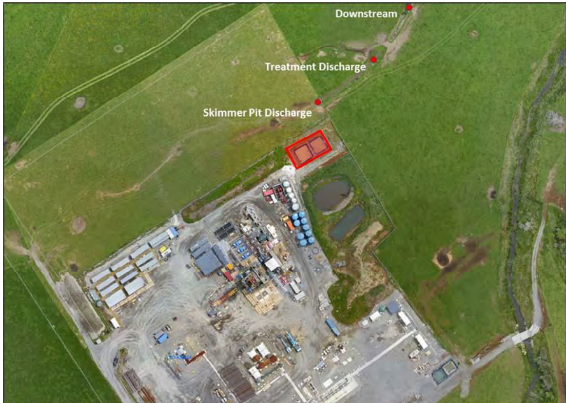
Figure 2 Aerial view of the Mangahewa-D wellsite showing the location of the skimmer pits (in red) and the discharge and downstream sampling locations.
