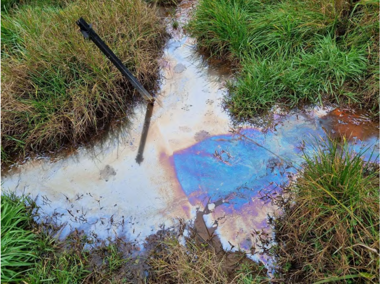
Photo 4 An example of the oily sheen as seen in the discharge next to the silt fences
