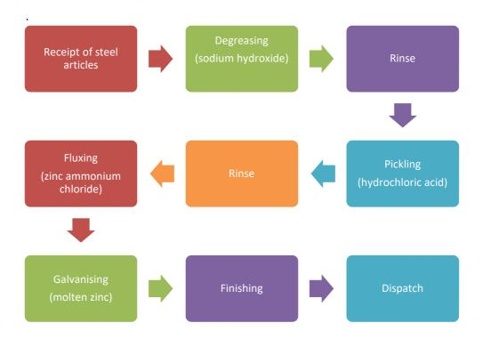
Figure 2 Hot-dip galvanising process undertaken at Taranaki Galvanizers
