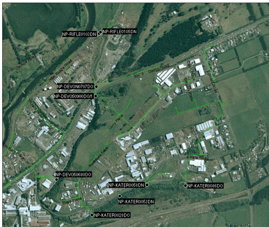
Figure 15 NPDC stormwater drainage and consented discharge points to the Mangaone Stream
