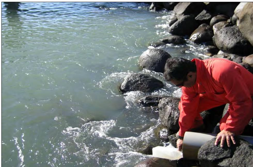
**Photo 4** Collecting a stormwater sample
