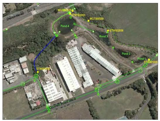
Figure 5 NPDC stormwater flow paths and sampling points
