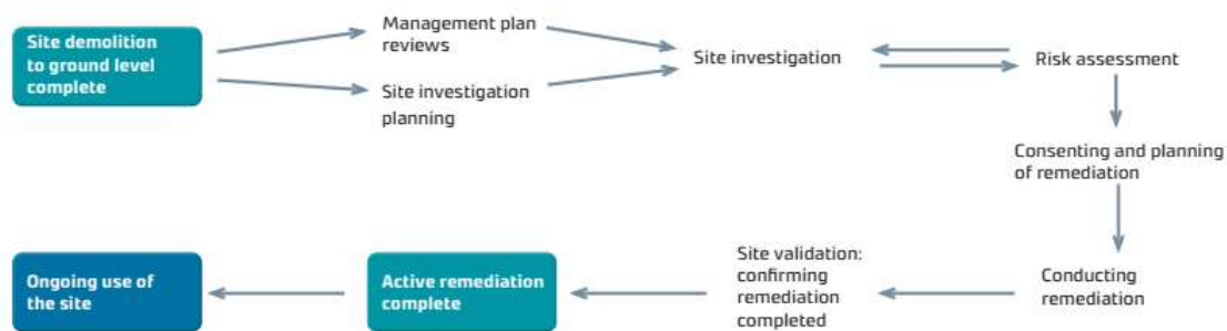
Figure 3: Conceptual framework for the remediation of the Dow Paritūtū site, as set out in the Draft Remediation Road Map for Discussion – Overview by Tonkin+Taylor.
