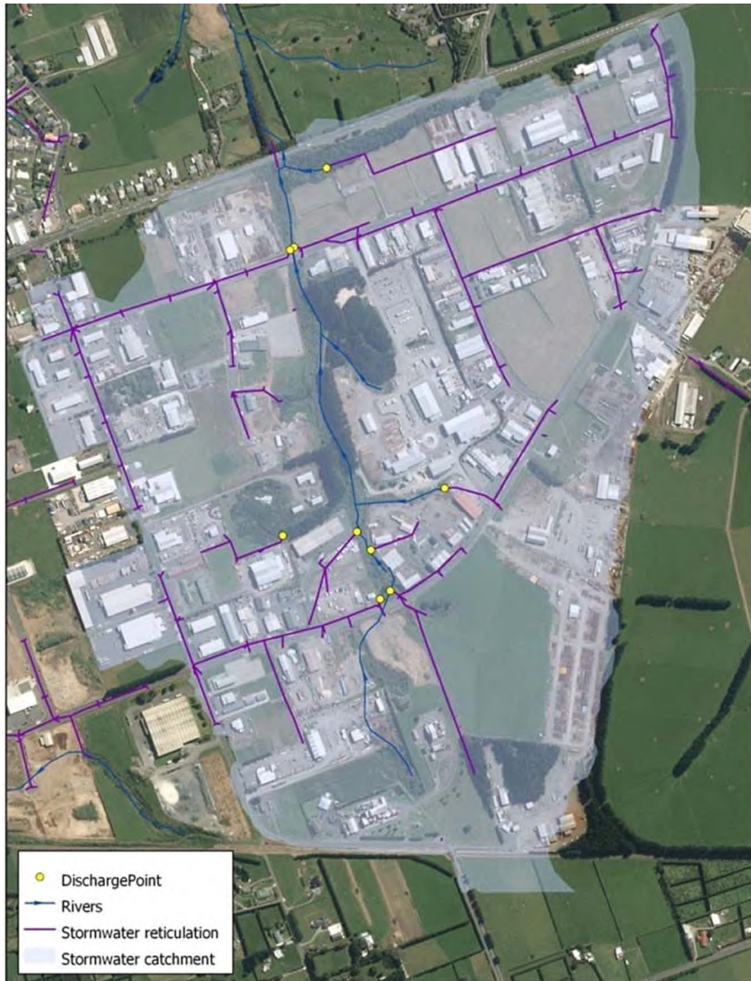
Figure 9 NPDC stormwater catchment, reticulation, and discharge points
