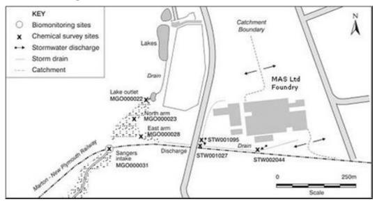
Figure 1 MASL foundry site, showing the boundary between Mangaone and Mangati Stream catchments and water monitoring sites
