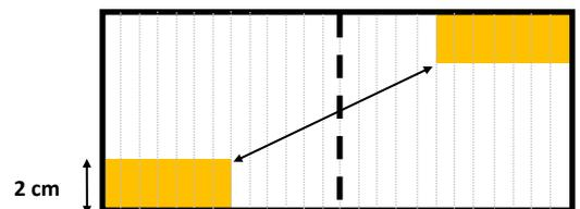
**Step 4:** Fold the card in half and pierce a 50mm flathead nail about 10mm from the centrefold on the top, and closer to the centrefold on the bottom half. This will set the card at 90° with an open mouth
