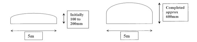
The process involves an extended period of standard aerobic composting conditions over a minimum of 35-40 days. The temperatures for worm processing are a lot lower than that of Greenwaste composting and should range between  $20^{\circ}-30^{\circ}$  Celsius. The process is
