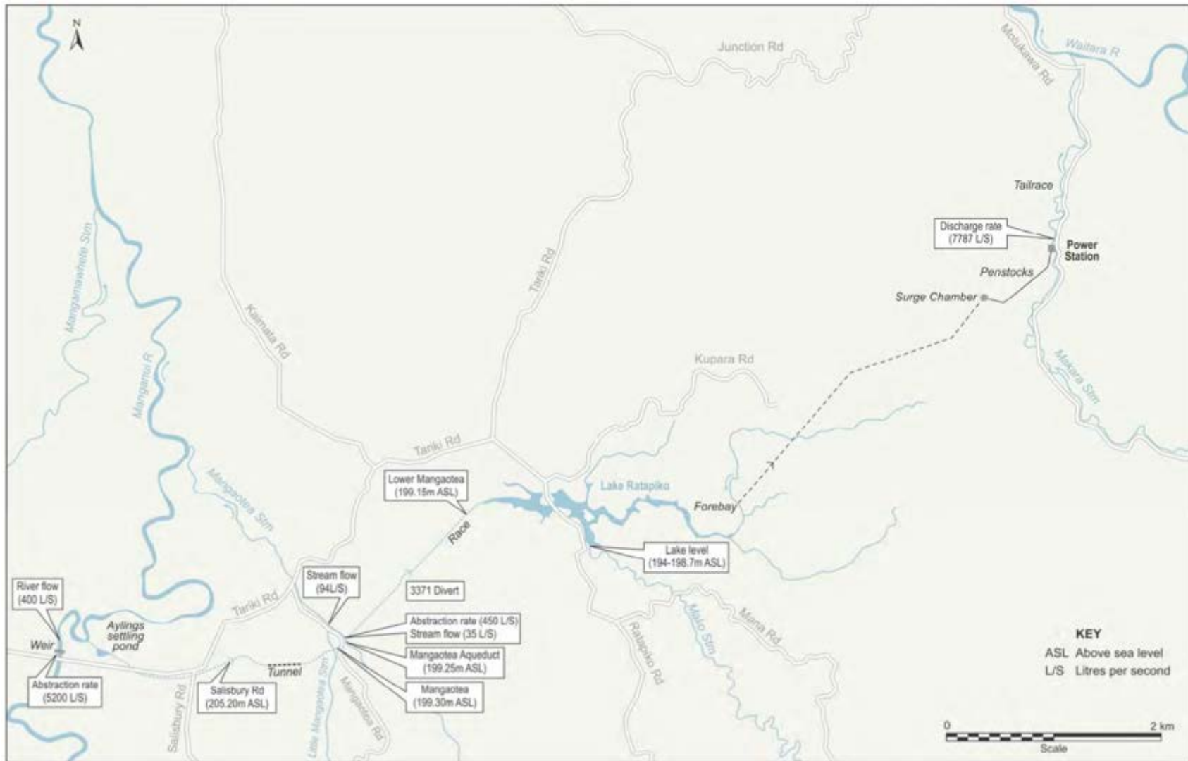
Figure 1.1. Location map of structures and surface waters associated with the Motukawa HEPS (from TRC 2020b).
