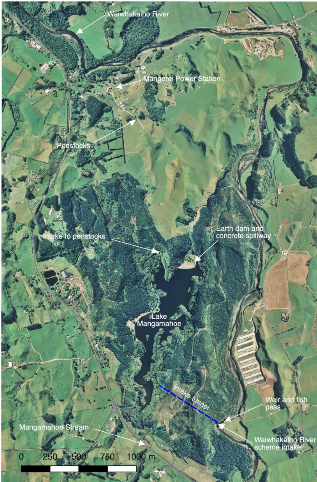
Figure 1.1. Aerial map showing location of structures and surface waters associated with the Mangorei HEPS.
