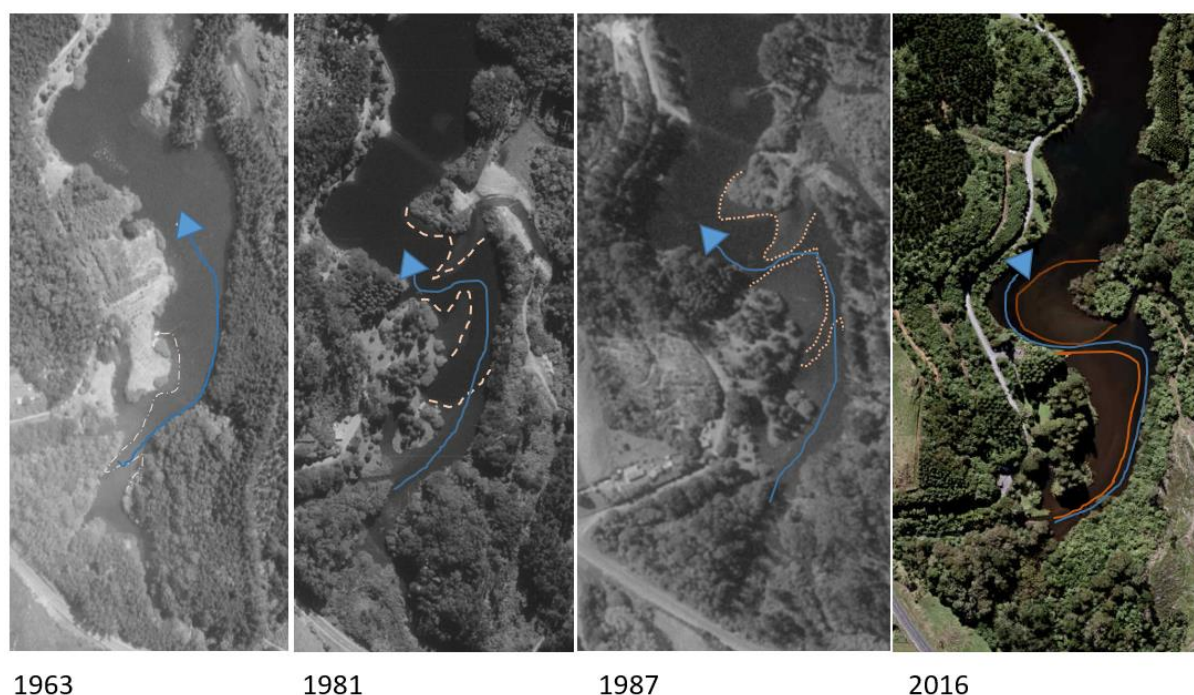
Figure 5.4: Sediment lobe/bar evolution through time (as denoted by the beige/orange lines) and the position of the Mangamahoe/Kent Road channel (as denoted by the blue line) through the southern arm of Lake Mangamahoe between 1963 and 2016.
