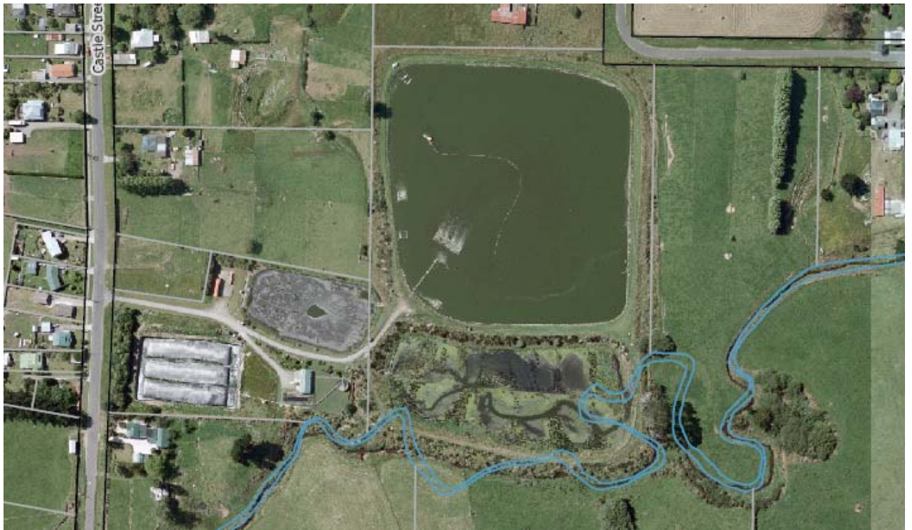
Figure 2 Aerial view of the Eltham WWTP showing the sludge geo-textile bags disposal area (lower LH corner) near the plant entrance
