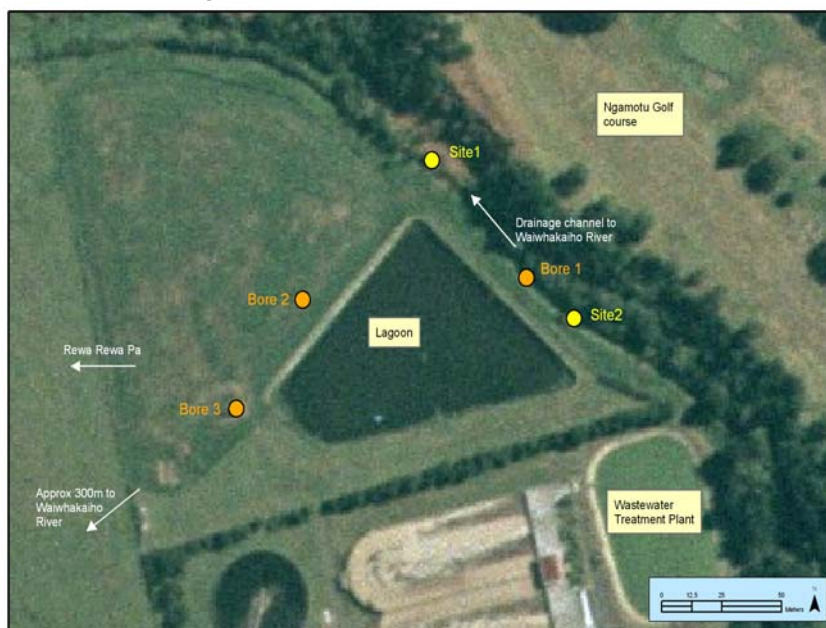
Figure 2 Site diagram of sludge lagoon showing location of NPDC's groundwater bore and drain sampling sites
